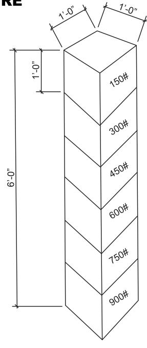
CONCRETE PLACED AT 6'-0" PER HOUR @ 70° F. CONCRETE TEMP.
